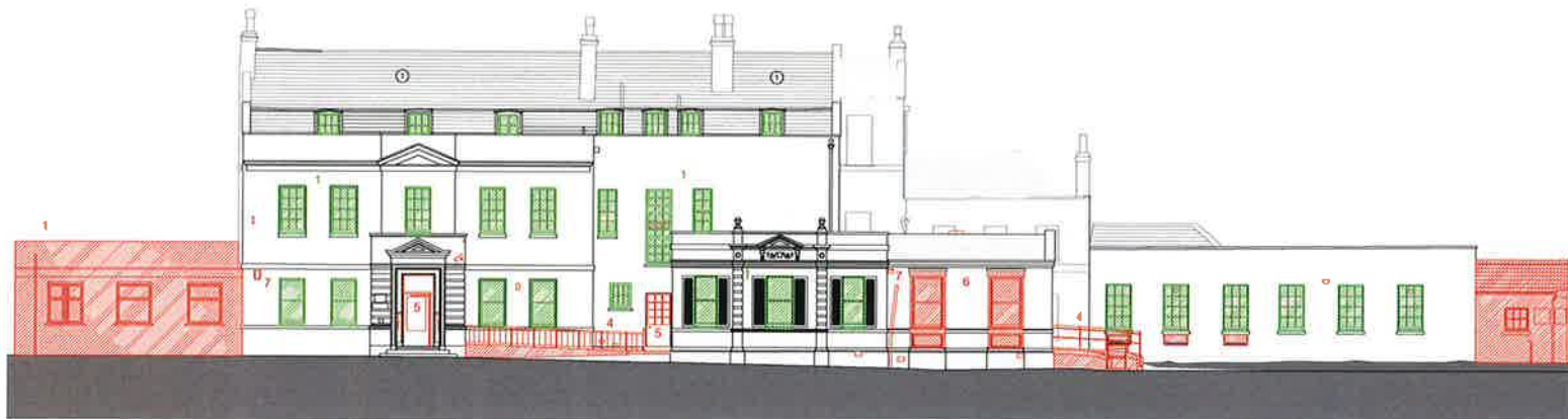
01 Demolition South West Elevation 1:100
